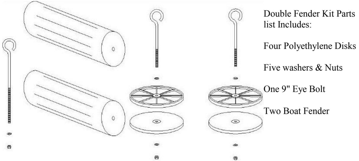
Place top disk over recess hole and run eye bolt through top disk hole through bottom disk hole. then use washers and lock nuts to tighten eye bolt & disk assembly.
